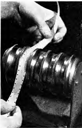
Fig. 2. Width gauge for use in factory.
